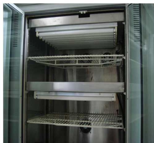
Fig. 1. Device for photodegradation of Pyr on soil surfaces.
